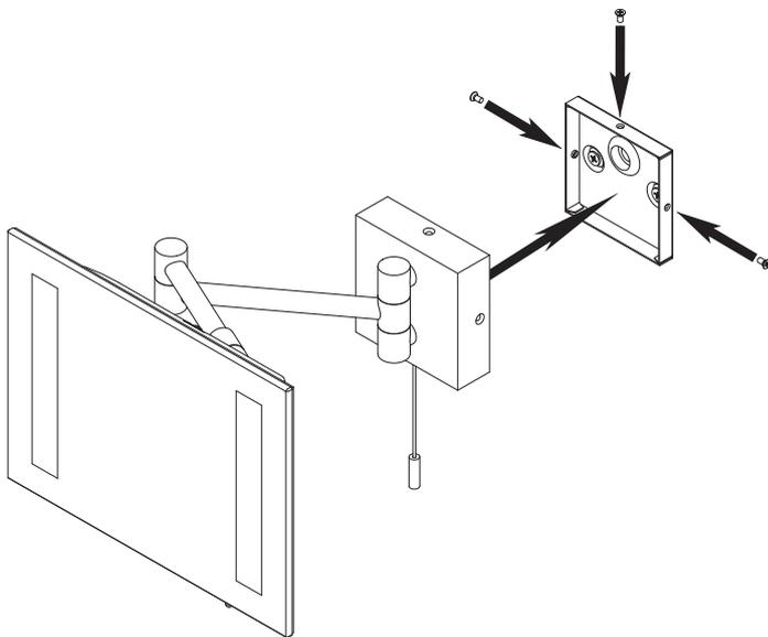
The swivel holding the mirror rotates through 340 degrees only.
